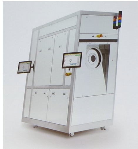
The PERC machines can handle 2-12 inches wafers
